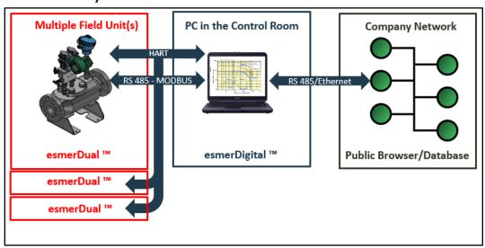
For wiring, a 24V cable and an RS485 digital cable is required between the field unit(s) and the PC in the control room. I/O tasks, including network connection for output, are implemented on the RS485- Ethernet- Modbus platform. Multiple field units can be controlled from a single PC in the control room.
